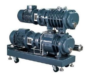
VPA-SSRT1300 is the combination of two vacuum pumps. VPA-SS180, which is water cooled dry screw vacuum pump and VPA-RT1500, which is air cooled Roots vacuum pump. This system can create higher pumping speed with higher vacuum (lower pressure). VPA-SSRT1300 is water cooled.
