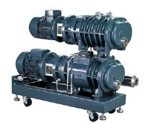
VPA-SSRT1800 is the combination of two vacuum pumps. VPA-SS180 which is water cooled dry screw vacuum pump and VPA-RT2000, which is air cooled Roots vacuum pump. This system creates higher pumping speed with higher vacuum (lower pressure). This system is water cooled.
