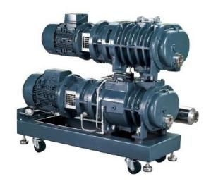
VPA-SSRT700 is the combination of two vacuum pumps. VPA-SS100, which is water cooled dry screw vacuum pump and VPA-RT900, which is air cooled roots vacuum pump. This system can create higher pumping speed with higher vacuum (lower pressure). VPA-SSRT700 is water cooled.
