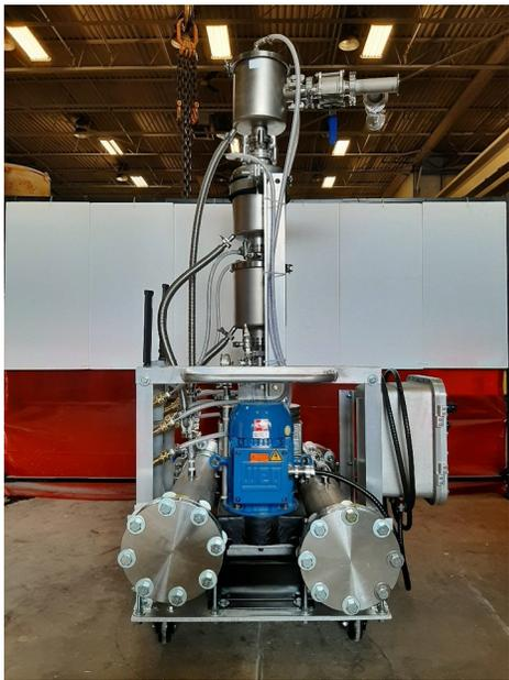
VPA-VSS60/Ex/SUS/SYS Process Vacuum Pumping Station with Explosion Proof Motor, Water Cooled Heat Exchangers, Reservoirs, Inlet and Exhaust Nitrogen Gas Purge valves, cooling water control and temperature controls.
